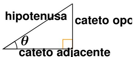
$$\begin{aligned}\operatorname{sen} \theta &= \frac{\text{cateto oposto}}{\text{hipotenusa}} \\ \operatorname{cos} \theta &= \frac{\text{cateto adjacente}}{\text{hipotenusa}} \\ \operatorname{tg} \theta &= \frac{\text{cateto oposto}}{\text{cateto adjacente}}\end{aligned}$$
